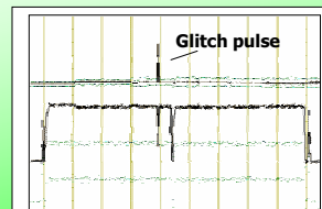
Power trace of a smart card being glitched during an RSA operation
